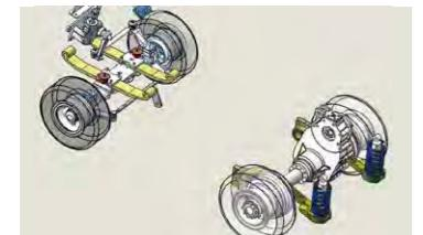
The front and rear axles equipped with a flexible suspension system offer less vibration and good comfort.
