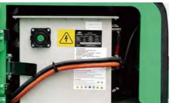
Removed from a side of the vehicle, the battery provided for the standard configuration can be replaced and maintained more easily and is applicable to continuous operating conditions.
