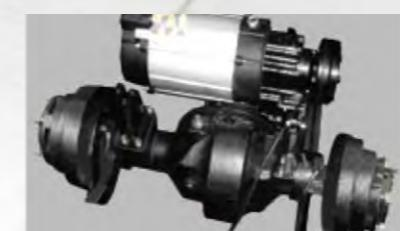
The world's leading horizontally-placed drive unit uses a special speed reducer with a large speed reduction ratio.
